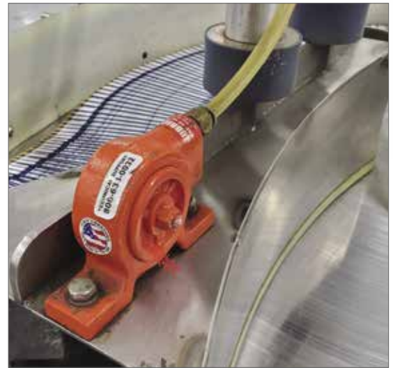
This pneumatic ball vibrator is used to keep this product line moving efficiently.
