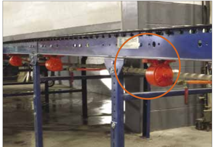
Material conveying systems work more efficiently with our Model VS Turbine mounted to structural members. Use one of VIBCO's complete mounting systems to get full efficiency and longer life from your vibrator.
