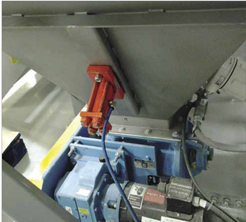
Above: Mounting this 50-2 unit (as seen on page 24). When mounted on a hopper it will help to create consistent flow of material. It aids in reducing overall batch times on the scale and in dispensing an accurately measured, consistent batch. No more labor time wasted banging on the hopper walls to release stuck material.
