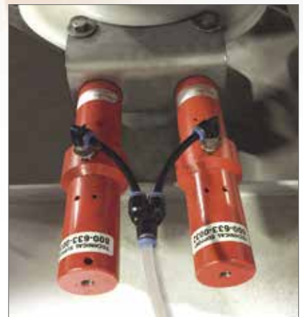
Vibrators used in tandem. All pneumatic piston vibrators require lubricated air for proper operation and long life. Low draw units like these 70-1's can share an air line and still run effectively.
