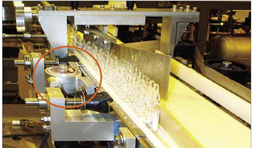
VIBCO's Model VS Turbine Vibrator works equally well on hopper applications or in conveying delicate glass vaccine bottles as the VS-100 silent Turbine is doing (above) without breakage or getting stuck.
