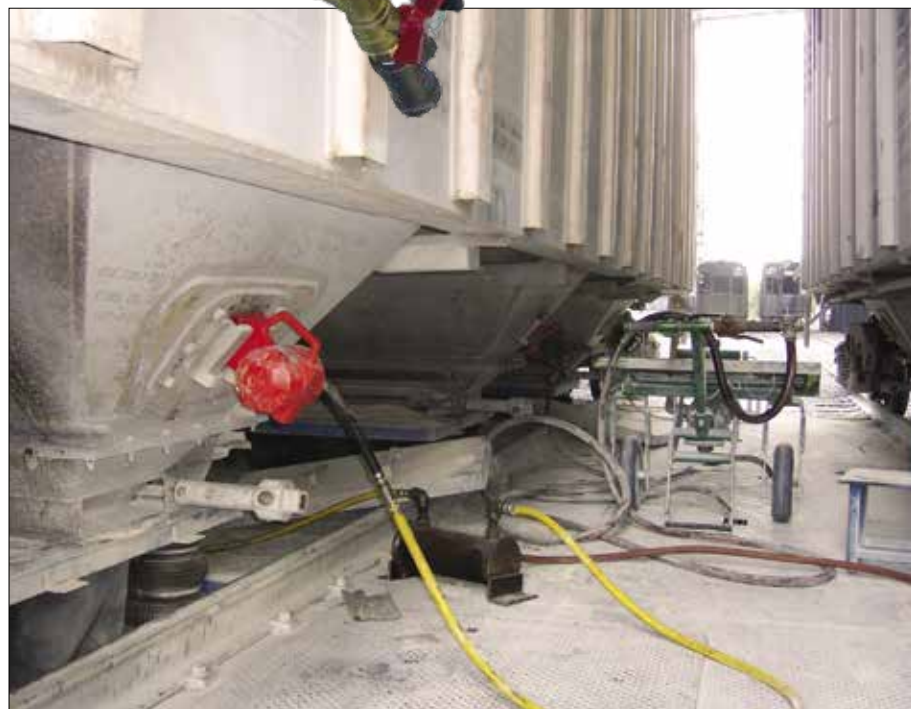
Vibration assists with material flowing into the railroad car as well as for unloading.
