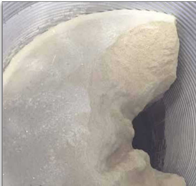
(above) Rathole created when grain sticks to the sides of the bin. Vibration breaks the static cling holding the grain in place.
